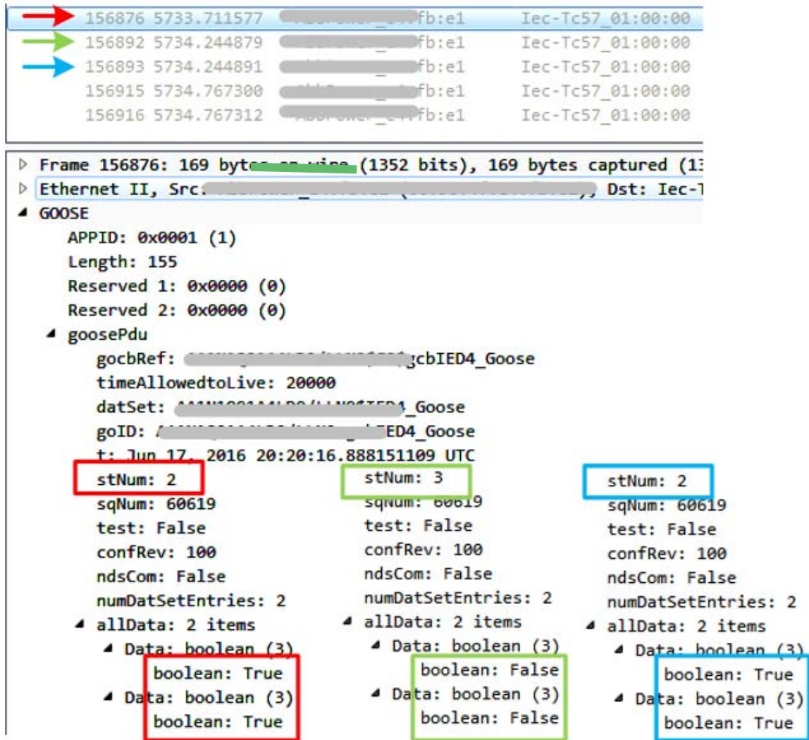
Figure 8. Wireshark Capture of Transmitted Messages (manufacturer’s details are intentionally omitted), red: original message with low status number, green: fake message with high status number, blue: original message retransmission with low status number.
