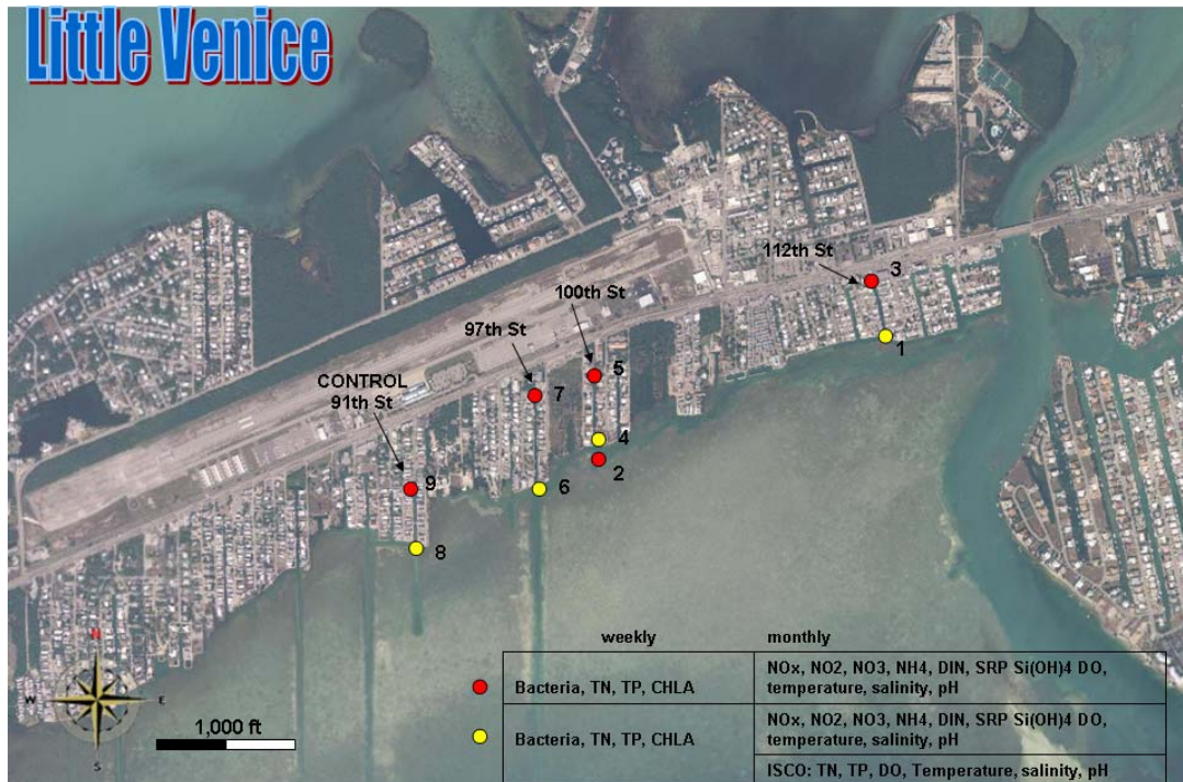
Figure 1. Little Venice Subdivision area in Marathon Key; sampling stations are shown. ISCO sampling is only performed bimonthly at yellow coded sites.
