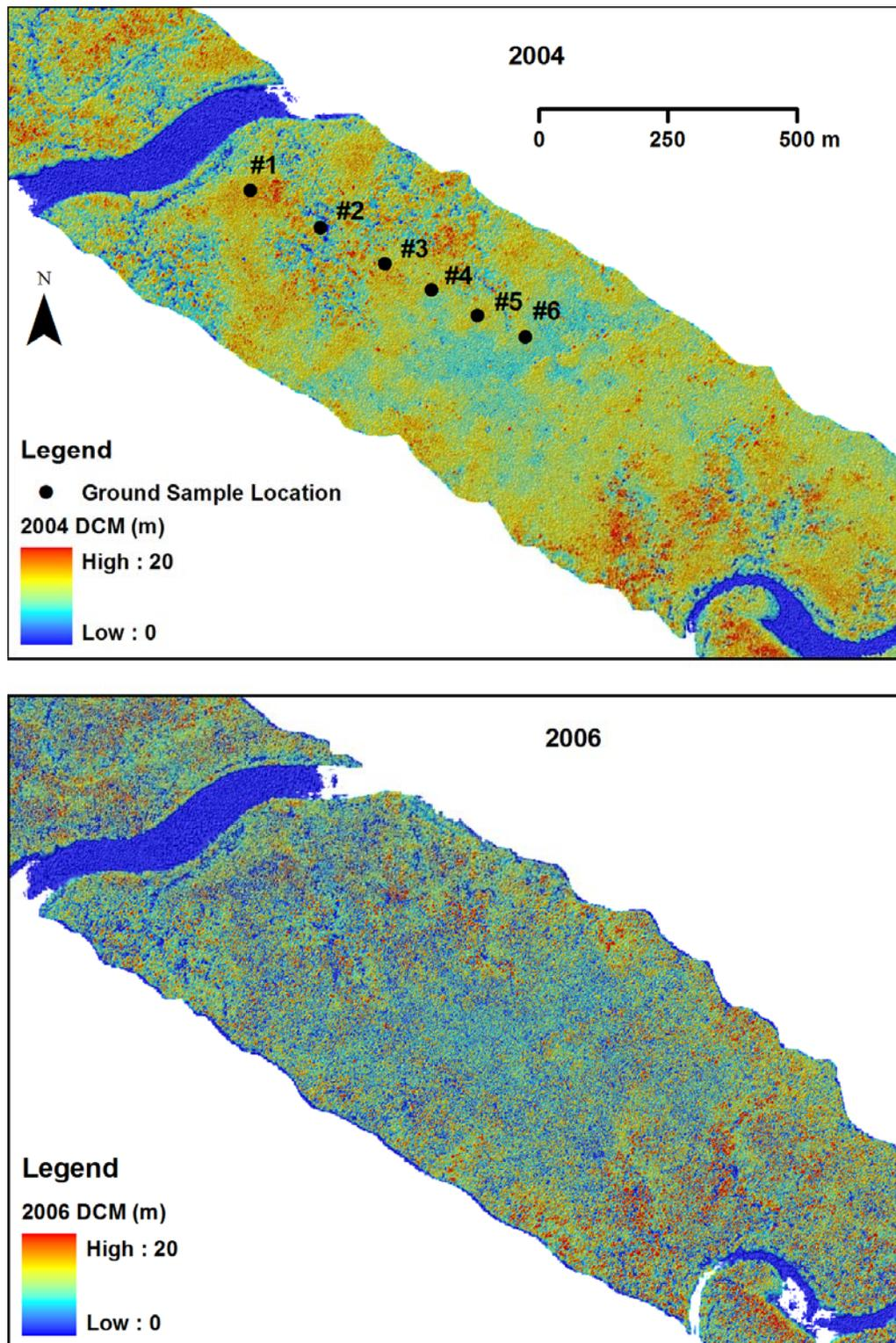
**Figure 10.** LIDAR derived canopy height distributions of 2004 and 2006 for plot 3 (a) and plot 6 (b) along a ground survey transect at the Broad River site.
