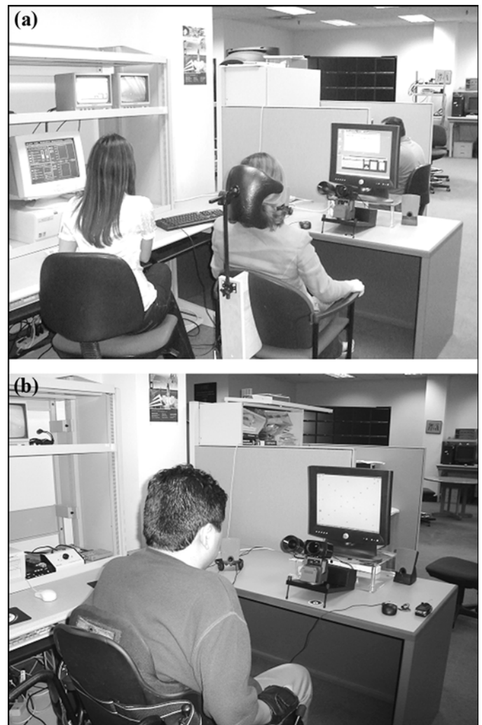
Figure 2. Eye-gaze-based human-computer interface setups. (a) Nondisabled subject using standard headrest to prevent abrupt head movement and (b) individual with motor disability in wheelchair.
