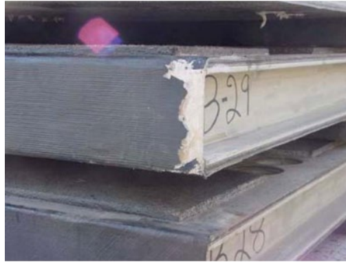
Figure 14 Fiber exposure (Telang et al. 2006)
