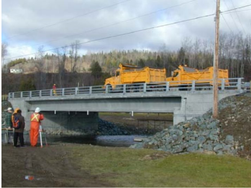
Figure 53 Deflection measurement (El-Salakawy, Kassem, and Benmokrane 2002)
