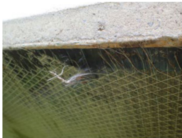
Figure 37 Fiber exposure (Baniya et al. 2022)
