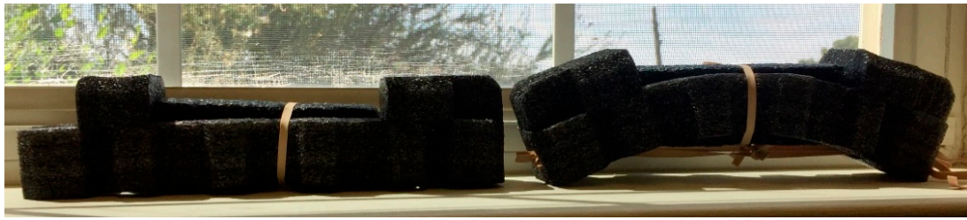
Figure 2. Prestressed plastic foam using rubber bands (on right) versus regular plastic foam beam (on left).
