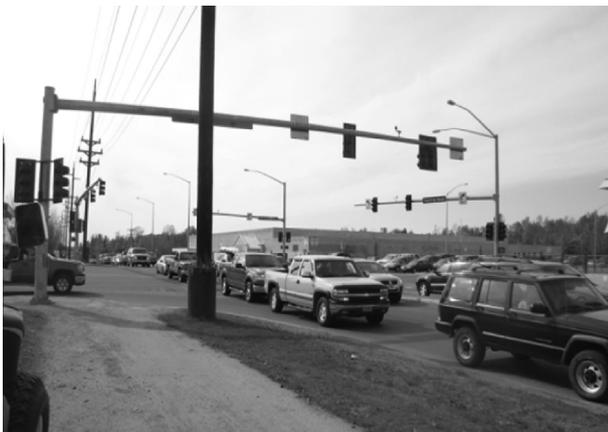
Fig. 3 – Picture showing the queue from the eastbound entrance approach blocking the upstream intersection on old Seward Highway and East Dowling Road.
