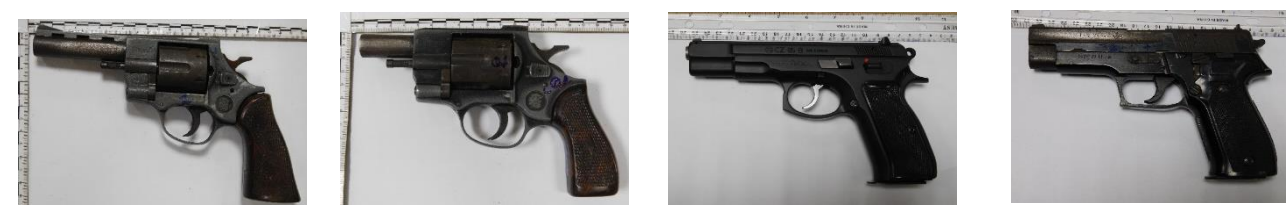
Figure 2: Firearms used: (A) Arminius Long barreled revolver (0.38 Special), (B) Arminius short barreled revolver (0.38 Special), (C) CZ Pistol (9x19 mm), (D) NP 22 pistol (9x19 mm).
