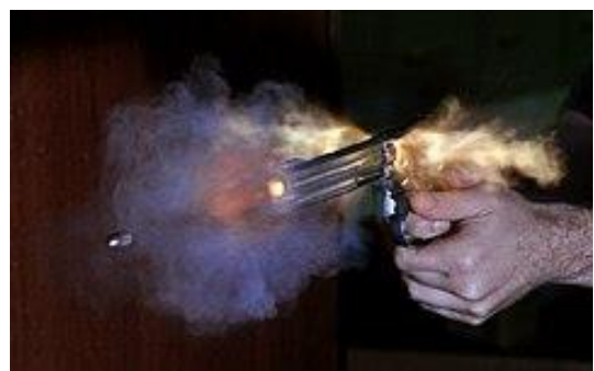
Figure 1: Expelling of GSR during a fire of a revolver
