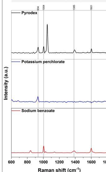
Fig. 6. SERS detection of Pyrodex gunpowder compared to  $\text{KClO}_4$  and  $\text{C}_6\text{H}_5\text{COONa}$  standards using the SPGE with gold deposited.
