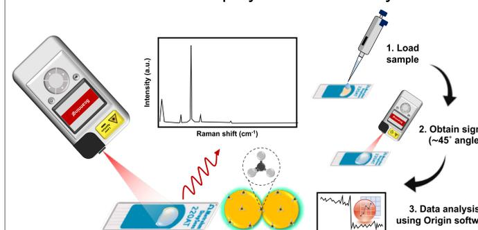
Fig. 4. Operating procedure for SERS detection using a Au-SPGE integrated with a portable SERS instrument.
