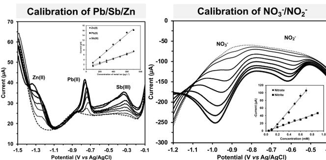
Fig. 2. SWASV detection of Zn, Pb, and Sb standards using the Au-SPCE and calibration.
