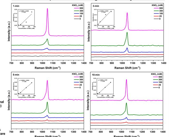
Fig. 5. SERS spectra with their calibrations obtained from detection of  $\text{KNO}_3$  in a concentration range of 0-500 mM at varying deposition times (1 to 10 min) of Au nanostructures on SPGEs via electrodeposition.
