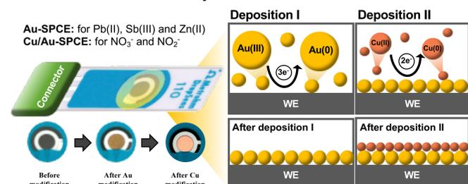
Fig. 1. Electrodeposition of Au(III) and Cu(II) on a SPCE
