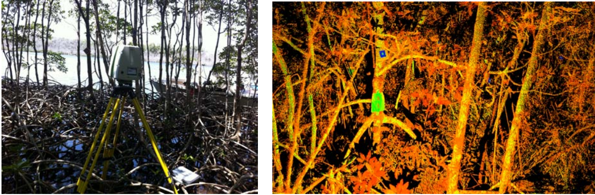
Figures 5.4a, 5.4b: Pictures of the intermediate size mangrove, SRS-5 site. On the left, the TLS scanner in the site. On the right, a LiDAR point cloud of the SRS-5 site.
