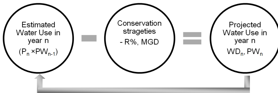
Figure 3.2 Sequential process in calculating desired water demand or per capita water use
