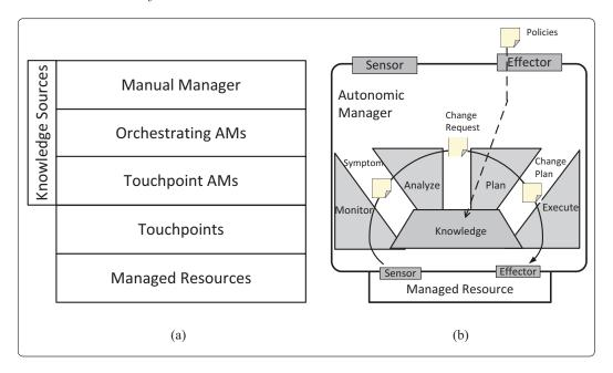
Figure 2.2: (a)AC Architecture (b)Design of a Autonomic Manager
