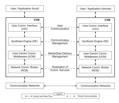
Figure 2.3: Layered architecture of the CVM.
