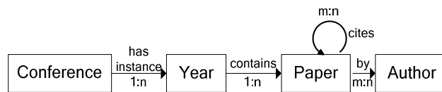
Figure 4: The DBLP schema graph.
