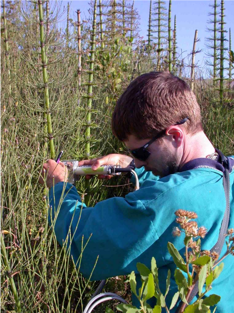
Figure 4.3 Measurement of stomatal conductance ( g_w ) of Equisetum giganteum stems with a steady state porometer in the Calatambo, Camiña Valley, Tarapacá Province, Northern Chile, March-May 2004.
