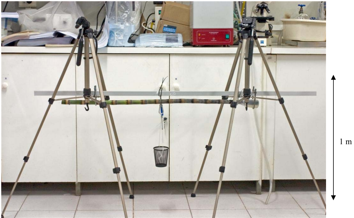
Figure 3.2 Three point bending apparatus for measuring flexural stiffness of giant Equisetum stems.
