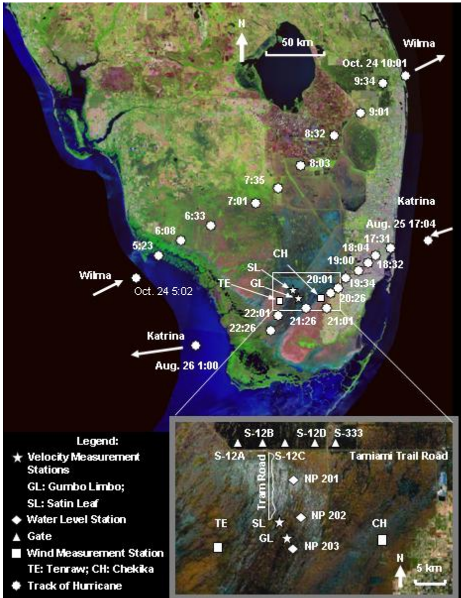
Figure 1 Hurricane tracks and locations of fixed Acoustical Doppler Velocity meters (ADV) and wind measurement stations. These locations include the fixed ADVs (GL and SL) and two closest wind measurement stations (TE and CH). Inset figure shows locations of gates and water level stations maintained by Everglades National Park.
